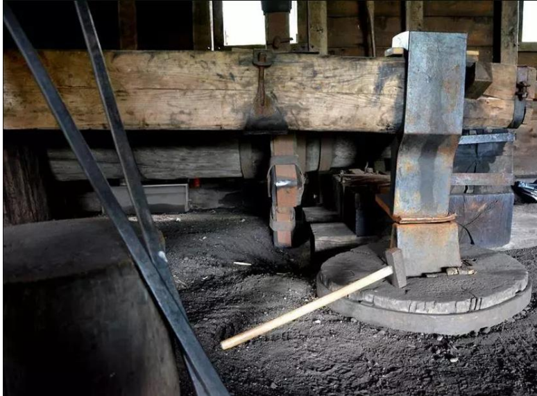
Reconstructed water-powered trip hammer at Saugus (photo credit: Saugus Iron Works National Historic Site)
